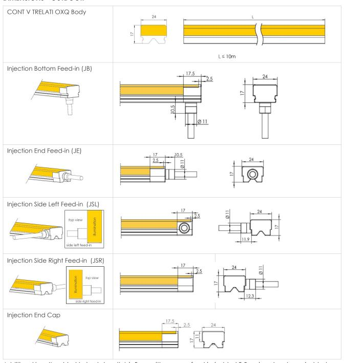
Additional length added to body length L is 5mm with any one feed-in (added 2.5mm) and end cap (added 2.5mm).
