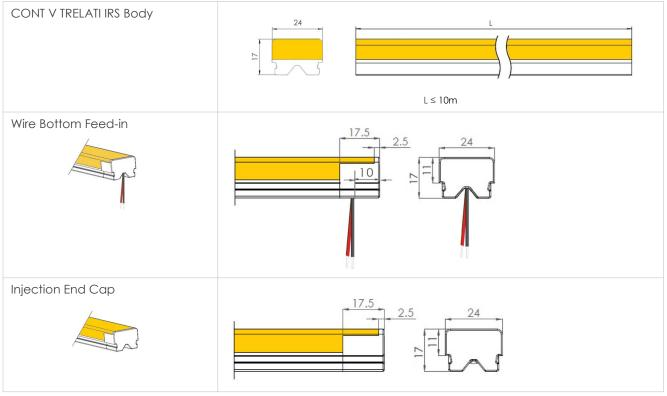
Additional length added to body length L is 5mm with any one feed-in (added 2.5mm) and end cap (added 2.5mm).
