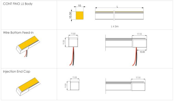
Additional length added to body length L is 5mm with any one feed-in (added 2.5mm) and end cap (added 2.5mm).
