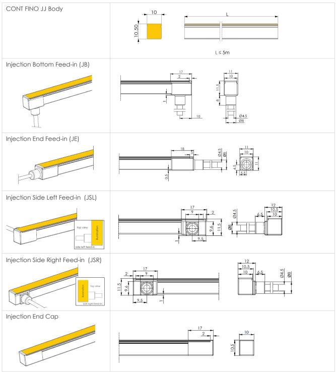
Additional length added to body length L is 5mm with feed-in (added 2.5mm) and end cap (added 2.5mm). Feed-in comes with 500mm feed-in wires.
